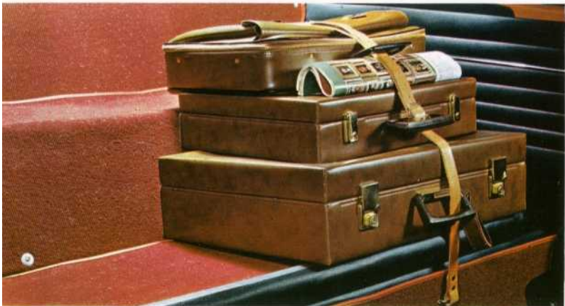
When the backrest is folded down this occasional seat forms a spacious platform for luggage.
